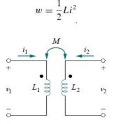
Consider the circuit above. We assume that currents  $i_1$  and  $i_2$  are zero initially, so that the energy stored in the coils is zero. If we let  $i_1$  increase from zero to  $I_1$  while maintaining  $i_2 = 0$ , the power in coil 1 is
