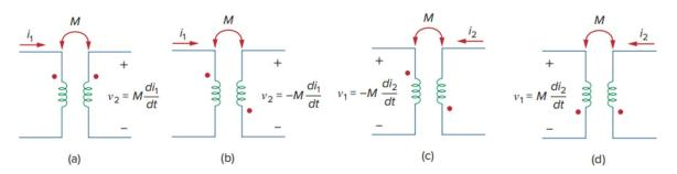
Given a circuit, the dots are already placed beside the coils so that we need not bother about how to place them. The dots are used along with the dot convention to determine the polarity of the mutual voltage. The dot convention is stated as follows:
